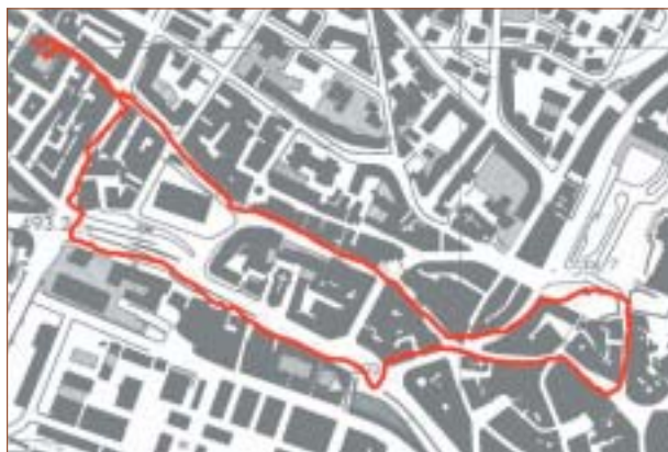
FIGURE 8 Pure DR navigation by a blind person in downtown Lausanne. The 1.9-kilometer path shows small discrepancies but reliably determines the real path followed. Bus power lines and parked cars negligibly influenced the computed trajectory.
